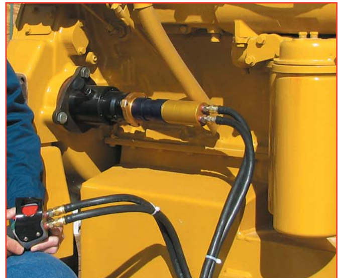
A B006PVR374-03-31P barring motor using pendant control, slow turning a Caterpillar 3408 engine.
