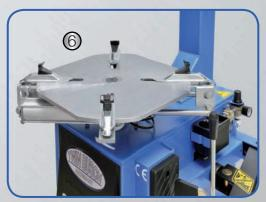
(1) Strong tyre press (2) Help-arm for professional use (3) Mounting head (4) Joystick for fine adjustment (5) Foot pedals (6) Special steel clamps | Large clamping diameter 10" - 24"
