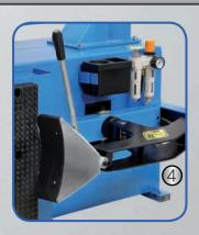
(1) Two help-arms for more efficiency (2) Air outlets in all clamping jaws (3) Large clamping range (4) Powerful bead breaker
