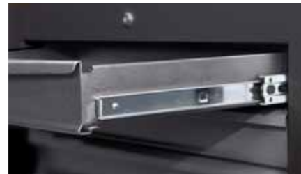
Auto returning ball bearing slider for smooth opening and closing. 50 kg drawer capacity
