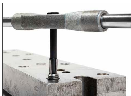
Spannen des Schraubenausdreher mittels Windeisen Setting the extractor with a tap wrench
