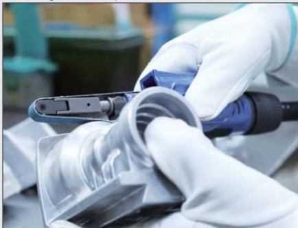
Deburring of die cast parts.
