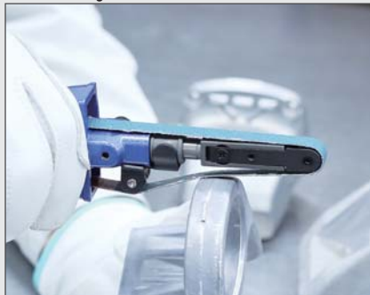
Detail finishing of aluminum material.
