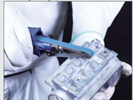
Chamfering of straight parts.
