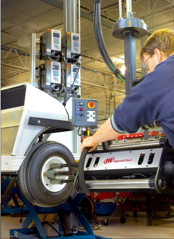
4-spindle horizontal/rotative DC fastening system
