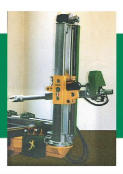
TRAXO REPLACES THE VERTICAL PULLING TOWER, BY UTILISING THE HORIZONTAL BASE OF THE TRADITIONAL ROTAX PULLER.
