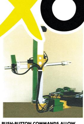
PUSH-BUTTON COMMANDS ALLOW MULTI-DIRECTIONAL MOVEMENT FROM THE HAND HELD CONTROL PANEL. THE OPERATOR IS FREE TO MOVE WHILE CONTROLLING THE ELECTRO HYDRAULIC PULLING TOWER AND OBSERVING THE REPAIR PROCESS.
