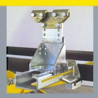
Sill clamp with extension plate for increased space between the vehicle and bench, ideal for use of measuring systems
