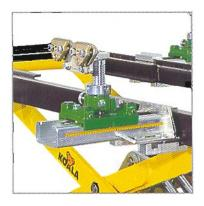
Possibility to utilise the McPherson overhead measuring bridge (E121) and the adjustable universal sill clamps with sliding base blocks of the GLOBALJIG Universal Jig System
