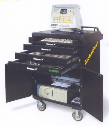
GlobalScan provides a graphic display of each vehicle, allowing the operator to compare the actual measurements with the precise vehicle specifications. Moreover, measuring several points in real time, it provides continuous updates during the course of the entire repair process.
