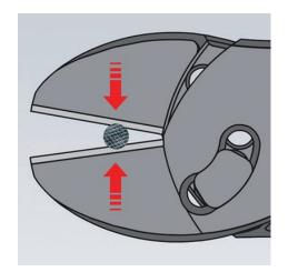
First make a notch in the wire using the KNIPEX TwinForce® until the required hand force increases considerably. Now open the pliers and slide the wire backwards towards the joint. Hold the cutting edge in the notches you have made in step 1.
