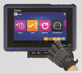
By using ultra-sensitive multi-touch technology the screen has been developed to respond effortlessly to touch, press and drag and it has been designed so that even gloved hands can use the IQVu.
